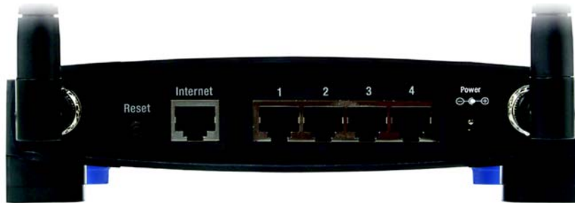
Figure 3-1: The Router's Back Panel
